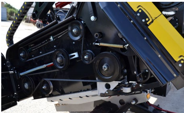
GEARBOX KNIFE BELT DRIVE
