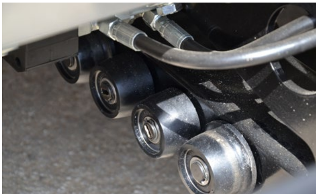
NEW ADJUSTABLE ROLLERS ON VARIO TABLE
