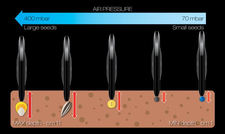
The airflow adjustment depends on:
