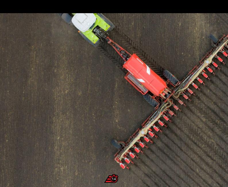
After exiting the distributor, the seed enters the new pneumatic system and it is transported into the ground through the air flow avoiding the negative bouncing effect. The seed counter is integrated on the seed tube and controls the seed delivery, while the soft rubber and self-cleaning press wheel holds the seed in the furrow, guaranteeing the best seeding accuracy and excellent depth consistency.
