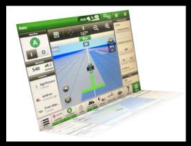
Once the prescription maps have been loaded into the ISOBUS monitor via USB, the tractor terminal obtains all the information regarding the rate of seed to deliver in each area.
