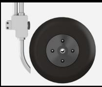
One electric motor for each seeding unit leads the transmission and controls the rotation of the seeding plate. After exiting the short tube, each seed is carefully blocked from the self-cleaning rubber press wheel.
