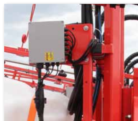
Control unit for management of hydraulic functions (OILDRIVE)
