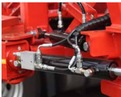
ALA opening jack with shock absorption system for side bumps
