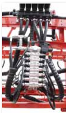
Oil-drive located inside the central unit
