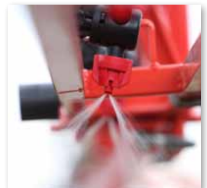
Nozzles protected inside the frame
