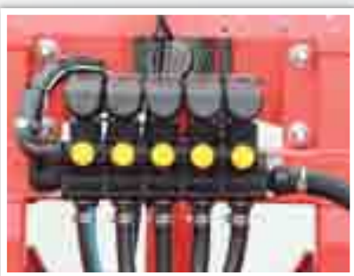
Electro-valves for boom sections control
