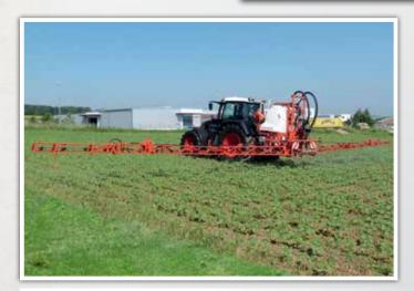
**TANK:** from 1300 to 1900 l **BOOM:** from 14 to 24 m
