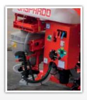
Gaspardo sprayers are built around the user's needs: the manual or electronically assisted control unit is designed to be very intuitive and ergonomic. All the levers of the main valves are placed in accessible positions or grouped together on a
