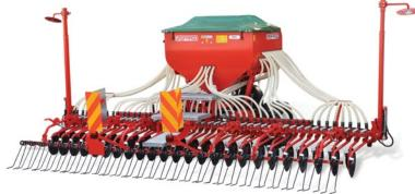
**PINTA 600** is the top range option: 6 m working width, heavy duty frame, 1500 I hopper and standard "GENIUS LITE" electronic transmission.
