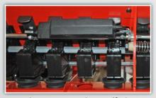
Distributor row shut off device for tramline system with remote control
