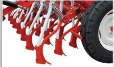
The units are arranged on 3 ranks to prevent soil or residue clogging. Each unit can express up to 50Kg of down-pressure thanks the robust spring load.
