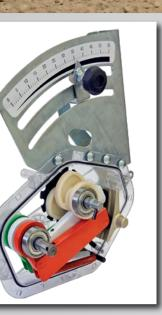
Our 3 cams gearbox makes the transmission of metering unit uniform and smooth. The use of ball bearings, confers greater resistance of the drive shafts. The lubrication system is an oil bath with inspection window. The calibration of the gearbox is fast and accurate.
