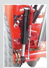
Hydraulic tensioning of centralized drill coulter bar.
