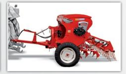
The trailed version is suitable for hilly lands or for tractors with limited lifting capacity.
