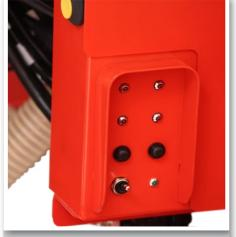
The easy access electronic control unit allows to calibrate the machine comfortably.
