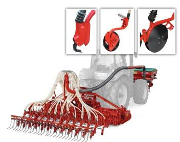
Seeding bar combinations are available either in "stand-alone" or "power harrow mounted" configurations. The **PA1 front hopper** offers 1100 I capacity, optimal weight distribution and no compromise on frontal visibility. After autumn seeding season, the hopper can be converted to the fertilizer distribution if combined to a precision vacuum planter.
