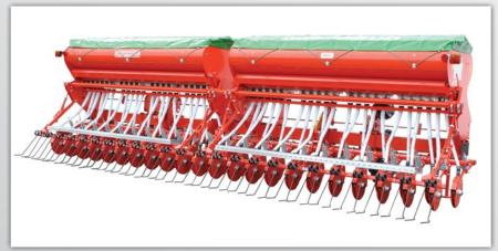
**MEGA** model is perfect for large extension on minimum tillage soils; working width 6 mt.
