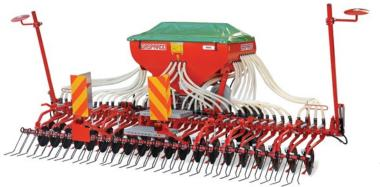
**PINTA** has a working width range from 4 to 5 mt and a 1000 lt hopper. Basic model has mechanical drive system; on demand is available the GENIUS LITE electric transmission.
