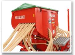
Hopper has a 1500 liter total capacity: 1000 for seed; 500 for fertilizer.
