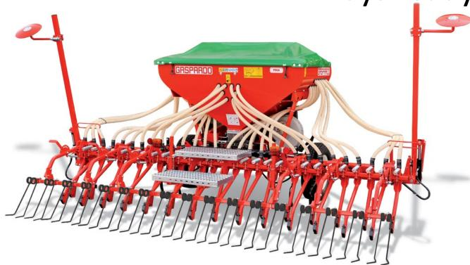
PINA is the compact option of the range. Hopper volume is 800 lt. Suitable for finely tilled soils.
