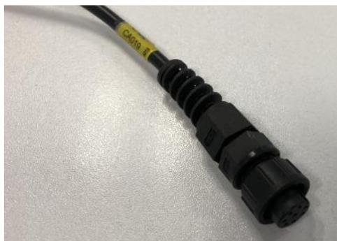
Connect cylindrical connector the display
