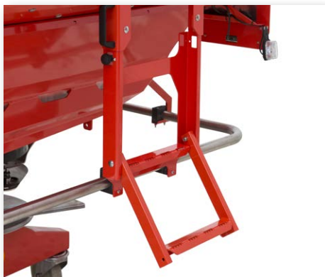
Ladder for hopper inspection
