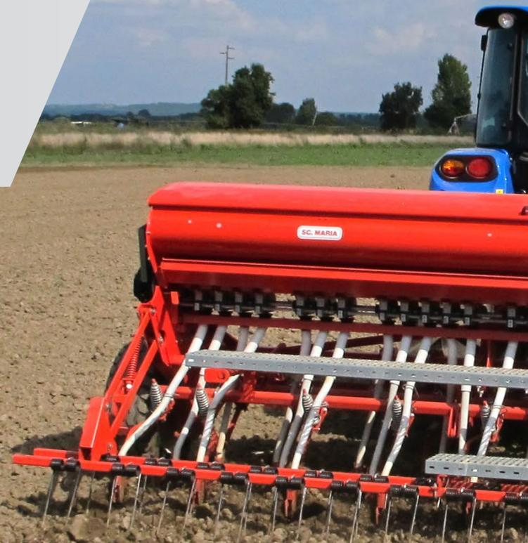
The seed distributor is composed by several elements to work at the best both with small seeds than with bigger seed. The contact spring feeler allows gentle seeds handling, while preserving the best vitality and the homogeneity of investment.
