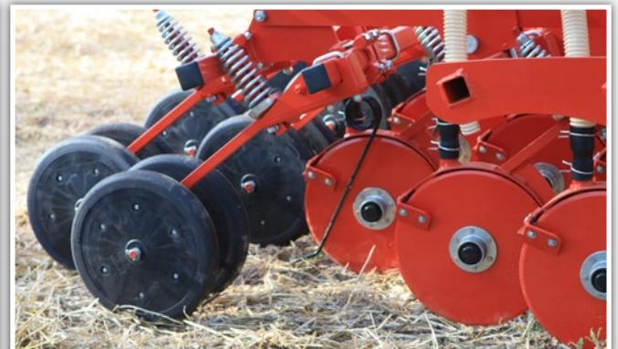
The seeding units are carried by a high clearance frame and arranged on 4 ranks to minimize, even at higher speeds, clogging of soil or crop residues. The seed covering harrow is available with straight or "S" type teeth and press wheels bar configuration.
