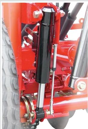
Hydraulic tensioning of centralized drill coulter bar.
