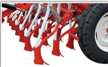
The units are arranged on 3 ranks to prevent soil or residue clogging. Each unit can express up to 50Kg of down-pressure thanks the robust spring load.
