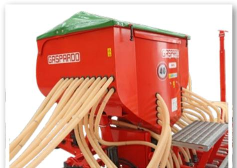
Hopper has a 1500 liter total capacity: 1000 for seed; 500 for fertilizer.
