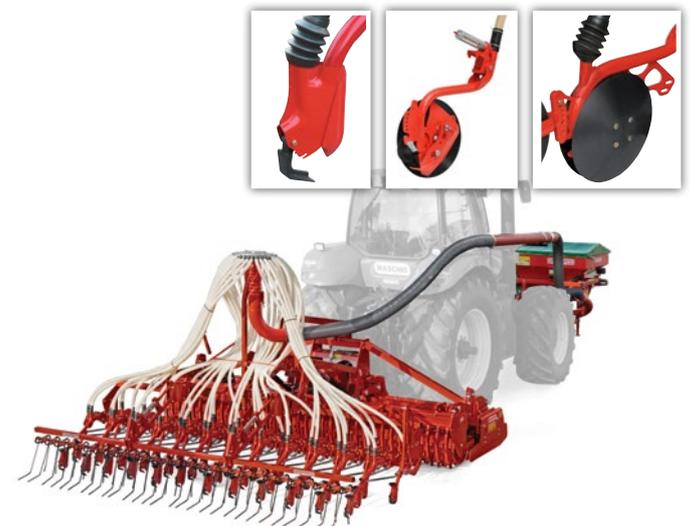
Seeding bar combinations are available either in "stand-alone" or "power harrow mounted" configurations. The **PA1 front hopper** offers 1100 l capacity, optimal weight distribution and no compromise on frontal visibility. After autumn seeding season, the hopper can be converted to the fertilizer distribution if combined to a precision vacuum planter.
