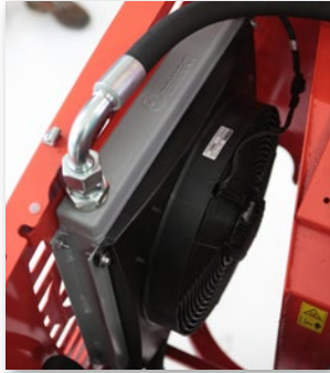
Hydraulic oil heat exchanger
