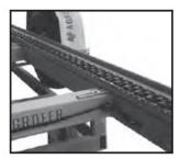
2 double wheel roll tracks for unloading "extra" bins for Mod: G4OTM RE - G40TM RS - ECO - ECO S (standard supply in all other models)
