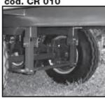
Axle with mechanical brake
