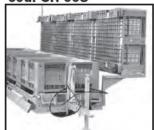
Structure for carrying the empty bins with "gate" opening and closing mechanism (for harvesting the tomatoes with a machine)
