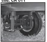
Axle with hydraulic brake, external cylinder and adjustment valve for brake. "Quick coupling operation of the tractor "
