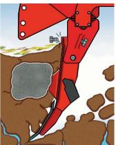
When the maximum load is exceeded, the breaking of the bolt allows the shank to be raised, avoiding possible damage to the shank and the frame.
